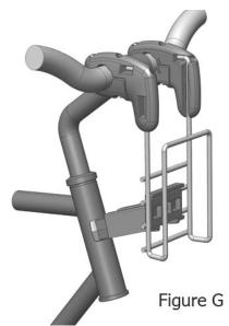
The basket can now be attached and removed from the bicycle quickly and easily (additional brackets are available for mounting on a second bicycle). Before riding with the basket, connect the two side safety straps around the handlebars and adjust the strap length to achieve a snug (not overly tight) fit. NOTE: Never ride with pets without fastening the safety straps.
