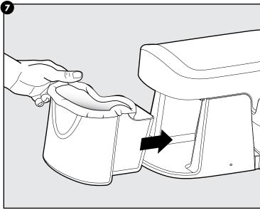
7. Use a plastic bag to line the waste bin. Insert the waste bin into the back of the litter box, making sure it is aligned and fully inserted into the unit. For additional help to minimise odours, add a small layer of clean litter and baking soda to the plastic waste bag or waste bin before placing it in the litter box.
