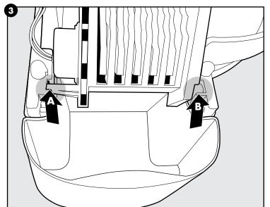
3. Next, install the conveyor by sliding the long post at the top (A) into the hole on the conveyor base. Then insert the short post (B) on the opposite side into the hole in the base by pressing it down into the hole with the L-shaped piece pointing down.
