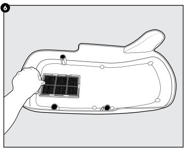
6. Place one carbon filter into the brackets on the inside of the conveyor cover. The black side of the filter should face outward. The carbon filter will help reduce odours from the waste bin area. Place the conveyor cover over the conveyor, making sure it is fully in place.
