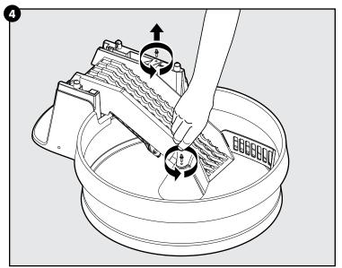
4. Remove the thumb screws from the center of the litter bowl and top of the conveyor. Lift the conveyor to its upright position.
