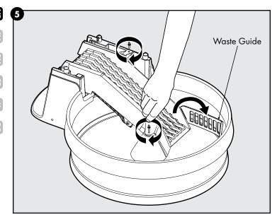
5. Lower the conveyor and tighten the thumb screws, then flip the waste guide down into place.
