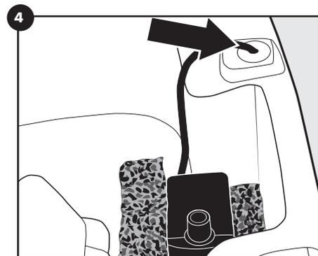
5. Attach the rubber connector to the pump tube if it is not already attached.
