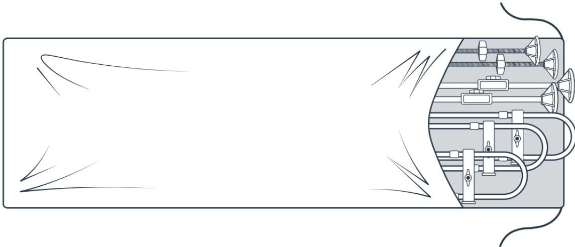
**EN** To store your barrier, simply press the blue buttons on each pair of clamps to remove the oval tubes from the upright supports. Twist the large wing nut on each support to release the tension holding the support in place. Remove the threaded rod from each hollow tube. Store these pieces in the included storage pouch until you're ready to use your barrier again.
