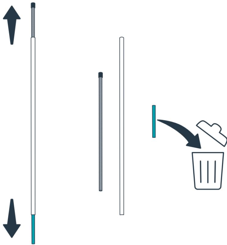
**EN** Remove the threaded rod and short, black plastic spacer from inside each of the two straight tubes. Discard the two plastic spacers.
