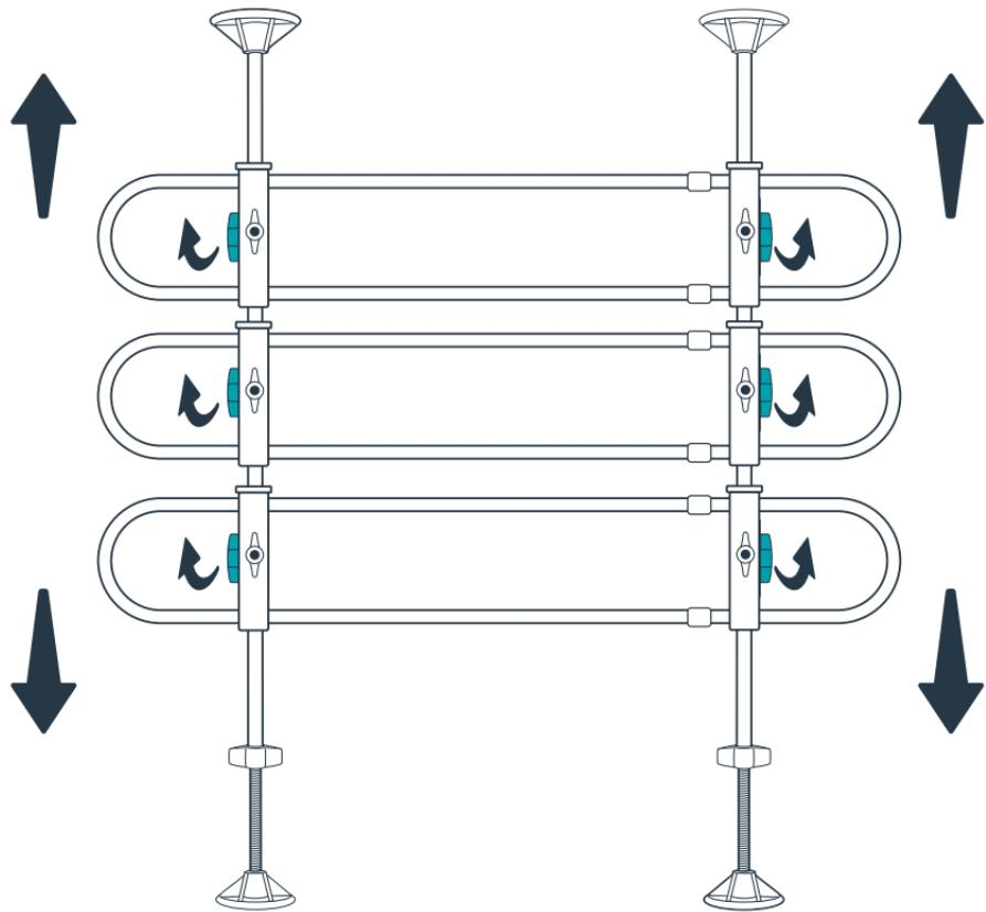
**EN** Now you're ready to adjust your barrier for a perfect fit! You can slide each oval tube up or down to fit your vehicle. Loosen the wing nuts on the mounting brackets to slide each oval tube up or down on the upright supports. When each oval tube is at the height you want, tighten the wing nuts on the mounting brackets.
