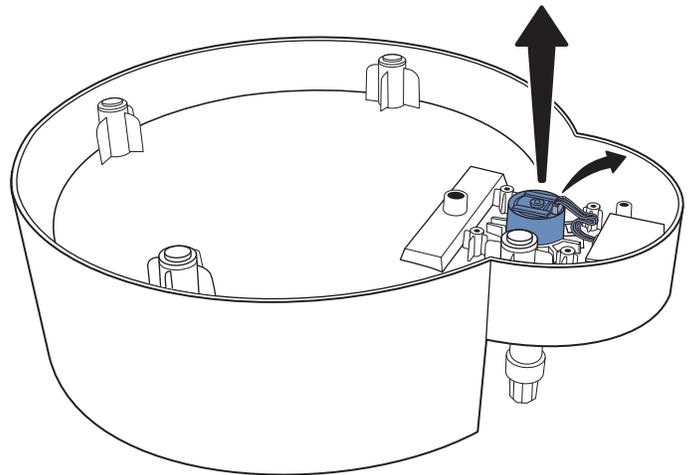
Carefully disconnect the ribbon cable from the motor. Lift the old motor out of the fountain base.
