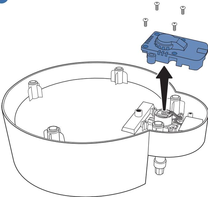
**Important:** Unplug the fountain before replacing the motor. Remove the bowl from the fountain base. Turn the fountain base upside down and place it on a table, making sure the stem is off the table edge.
