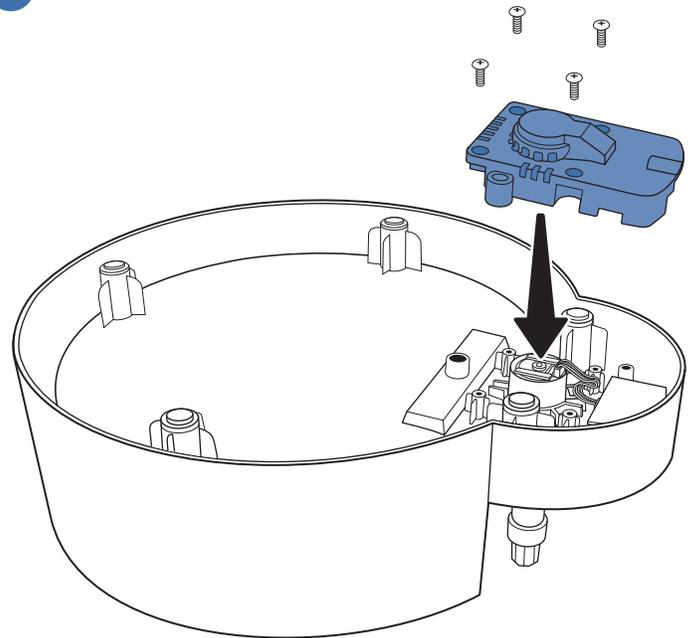
Replace the motor cover and secure it with the four screws you removed earlier.
