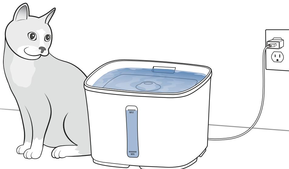
**EN** Place the fountain where your pet will use it. Fill the bowl with water up to the max fill line on the window and then fit the tray onto the top of the bowl. The outlet at the centre of the tray should connect with the tube on the pump housing.
