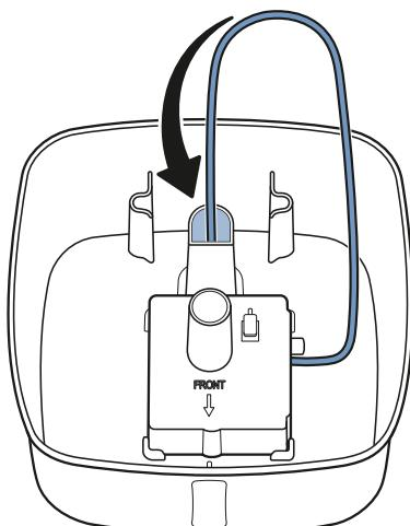
**EN** Insert the silicone cap and fold its top edge down over the top of the tube. This holds the cord in place and prevents leaks.
