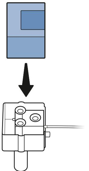
**EN** Place the foam filter around the faceplate of the pump inside the pump housing. The foam filter may be a tight fit inside the pump housing, but that is normal and will help keep the pump in place.
