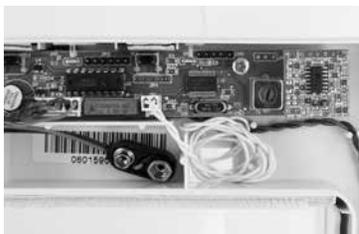
Attach the porch cable to the electronics board and hold the exterior and interior sections together using the two M6 screws. Tighten the screws to hold the Petporte smart flap® in the desired position within the opening.
