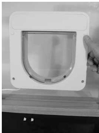
Once positioned, attach the large cover plate and secure with the four self-tapping fixing screws. Click in place the small cover plate. Place all of the blanking plugs, four small ones for the self-tapping fixing screws and two large blanking plugs for the M6 screws. Finally, power up your Petporte smart flap®.
