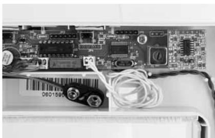
Attach the porch cable to the electronics board as shown. Any excess cable must be routed to the right of the battery compartment.
