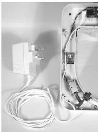
Attach the low voltage power supply connector to the electronics board and pass the power cable through the clips and out the opening at the bottom of the interior section.
