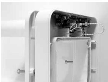
Temporarily attach the porch and exterior section to the interior section with the two M6 screws.
