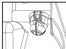
5. Hold these parts in place with one hand while attaching the Housing with the other hand (**Fig. 12**). Attach the Housing by sliding the cutout in the wall of the Housing down in between the Flow Control Knob and Intake Plate. The Housing will click into place, when the side tabs are inserted in the Bowl (**Fig. 13**).
