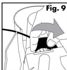
2. After turning the Pump a quarter turn, it should now be even with the bottom of the Bowl (**Fig. 9**). Turn the Bowl back over.
