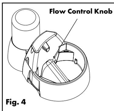
10. Set your desired flow rate with the Flow Control Knob, which is next to the ramp inside the Bowl. When the Flow Control Knob is in the 10 o'clock position, flow is at its lowest. When the Flow Control Knob is in the 2 o'clock position, flow is at its highest (**Fig. 4**).
