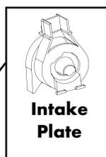
4. Join the Flow Control Knob and Intake Plate together by placing the tabs of the Flow Control Knob into the groove of the Intake Plate (**Fig. 11**).
