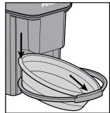
chute and tilting front of bowl forward, sliding under lip on holder. Lower back of bowl into place.
