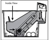
Lower back of conveyor and align with gear in hopper base. Push red conveyor latch to lock in place.
