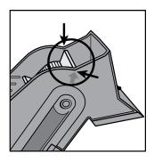
**To Install Conveyor:** Before installing conveyor, align one lip on conveyor belt with
