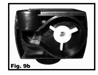
Once the stator is removed, you can remove the impeller (3 white-blade propeller). The impeller is held in place magnetically, simply get a fingernail underneath the plastic blade and lift out. (See Fig. 10)
