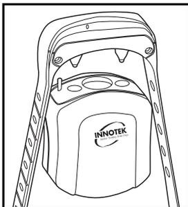
When you remove the collar from the charging station, the unit will automatically go into self-test mode for about 8 seconds. The collar's internal diagnostics will check that the battery charge is full and that all circuits are working correctly. Do not touch the
