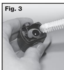
Clean with warm soapy water. Use a cotton swab or a small cleaning brush to get into the motor cavity and remove any build-up.
