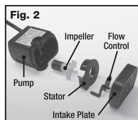
With your thumb and forefinger, gently squeeze the sides of intake plate, and pull off. Remove the flow control, stator and impeller. To remove impeller use a fingernail to lift out; it is held in magnetically.
