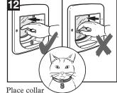
key on center of tunnel and push flap. Do not force flap open with magnet in hand. Fit hanging key to your cat's collar.
