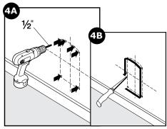
**4B.** Beginning in one of the holes you just drilled, carefully cut along drawn template lines using a jigsaw or other appropriate cutting device.
