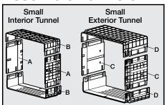
Note: Small Wall Entry Kit assembly does not require Step 3A. The tunnel sides (component A) of the Medium Passport™ Wall Entry Kit may be preassembled at the factory and may not require step 3A.
