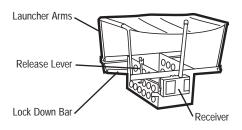
Manual launcher: Attach a pull cord (you provide) through the Pull Hole, and then to the bottom hole of the Release Lever. Pull the cord to release the launcher.
